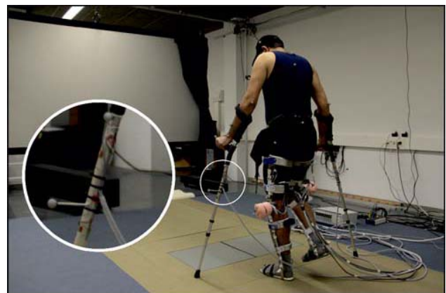
Fig. 1. Authors' ongoing project: development of active SCKAFO.
